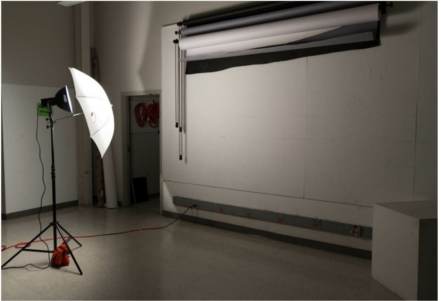
Umbrella in the diffusing arrangement. Note: Some of the light is reflected back and lost. The light toward the wall is reduced and scattered.
