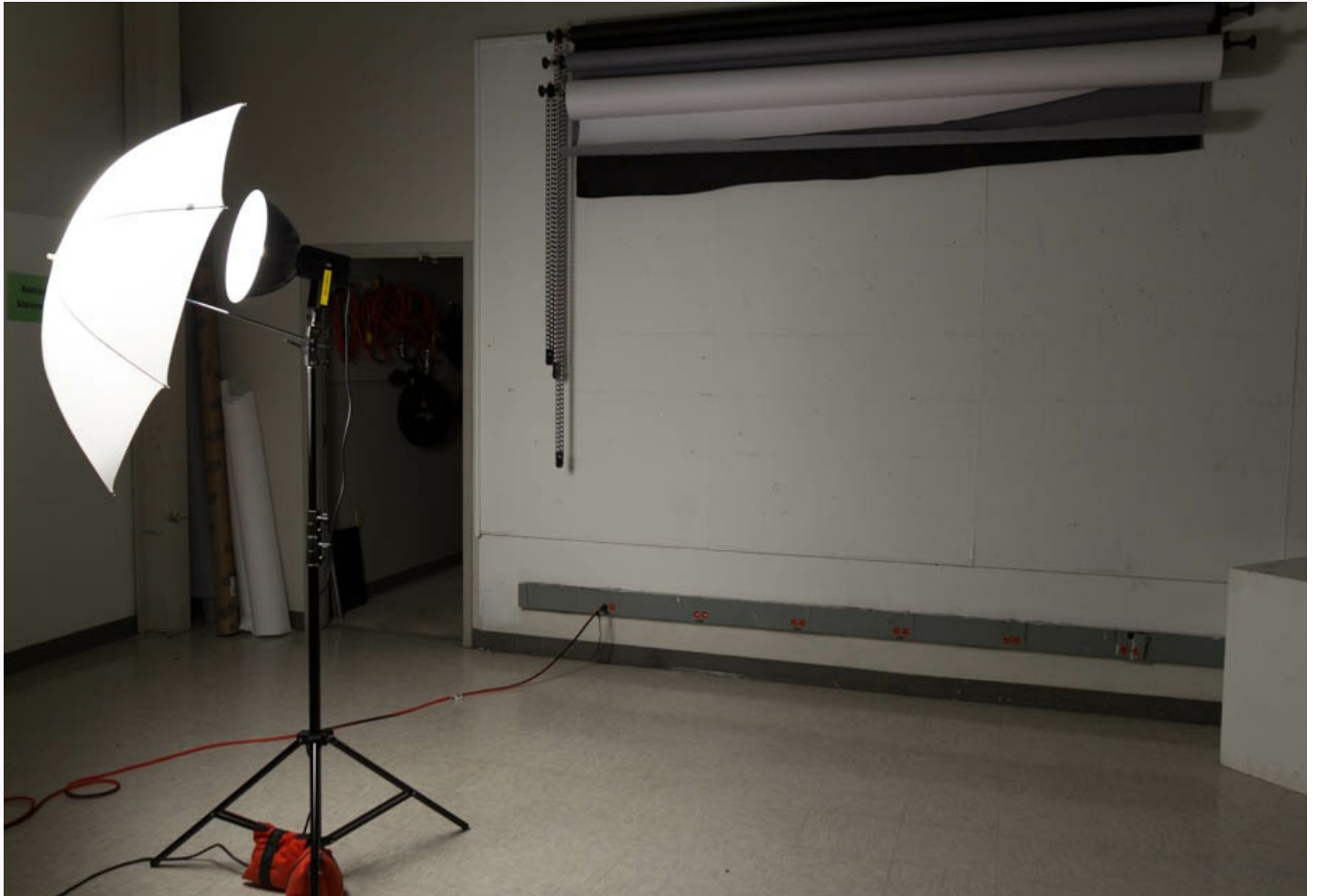
Umbrella set up as a reflector. Light on the wall is much more spread out and less intense. Note: The umbrella in the illustration is not a true reflecting umbrella because it lets light through it. It did have a shiny interior, so it did reflect some of the light.
