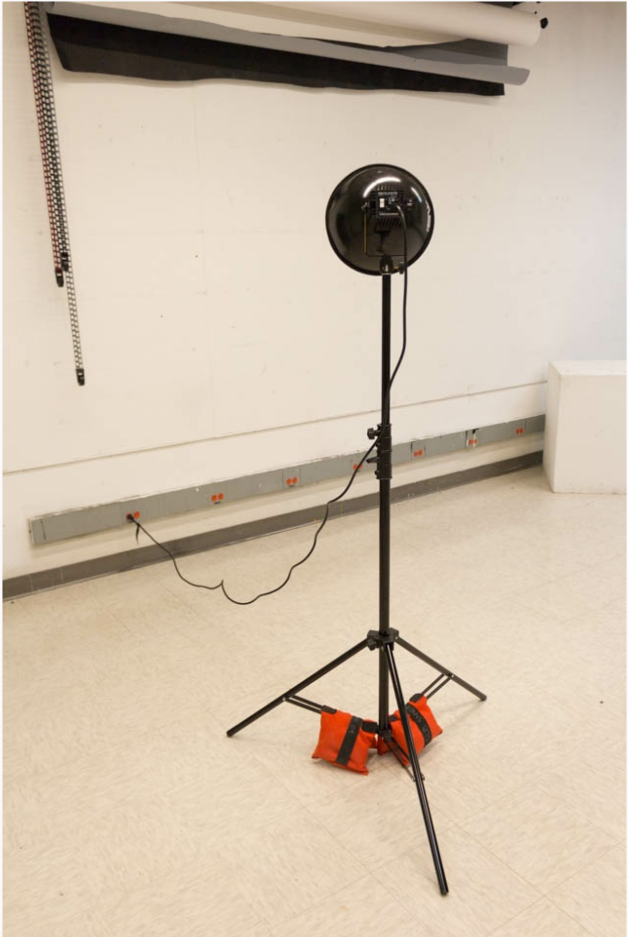
DO NOT ALLOW POWER CORDS TO DANGLE IN MID-AIR
