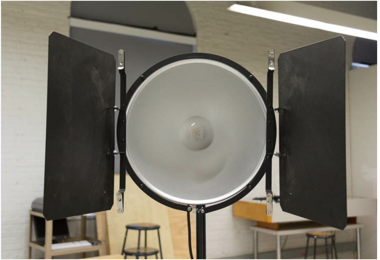
Barn doors on hot light
