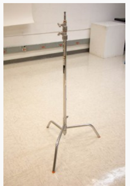
A C stand with its legs set up
