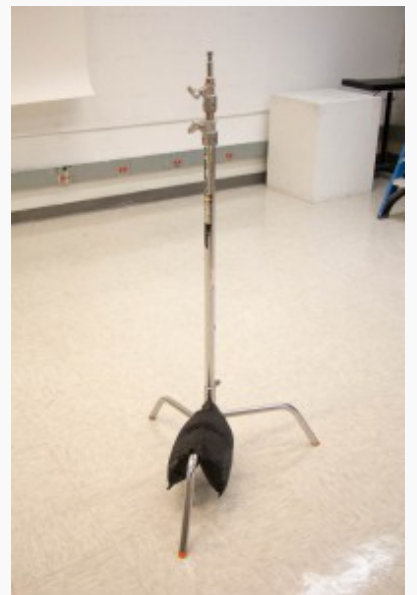
C stand with a sandbag to add stability
