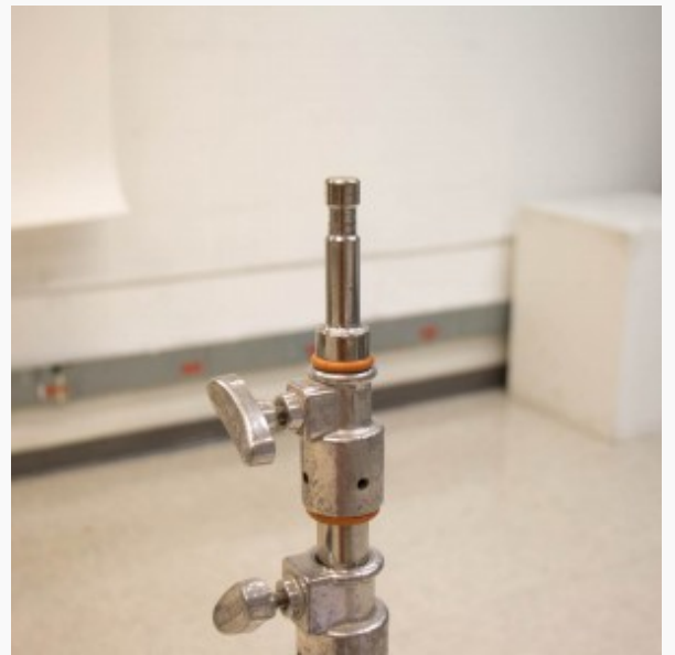
Mounting pin on a C stand
