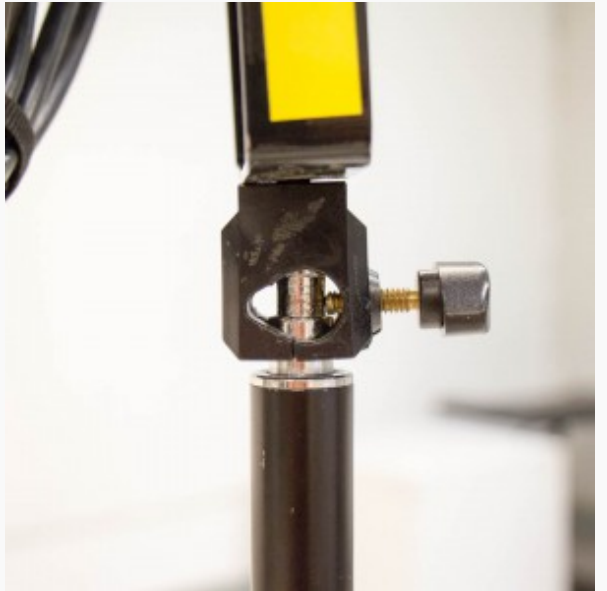
Do this! — Light mounting socket is fully seated and the screw is clamped in the notch in the pin
