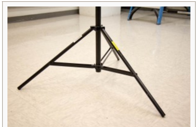
Studio stand with leg stance widened with stabilizing arms parallel with the floor
