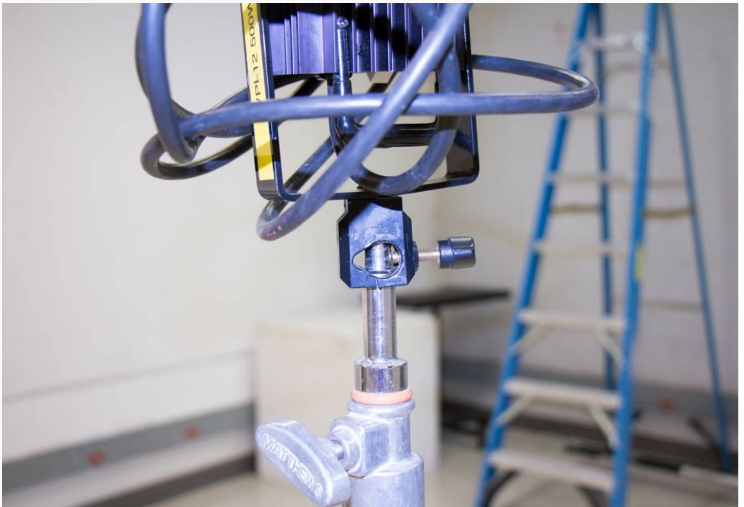
C stand with the mounting socket of a light firmly seated on the pin of the stand. The clamp screw is tightened into the groove on the pin.
